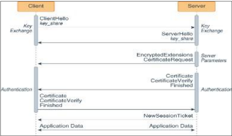
Figure 10 Transport Layer Security (TLS) Protocol Overview
