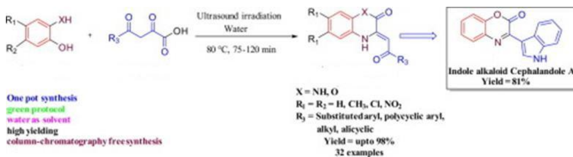
Scheme 7 Synthetic pathway for functionalized 2-oxo-benzo[1,4]oxazines
