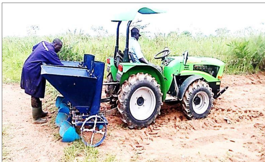
Figure 2 Planter mounted to tractor ready for planting
