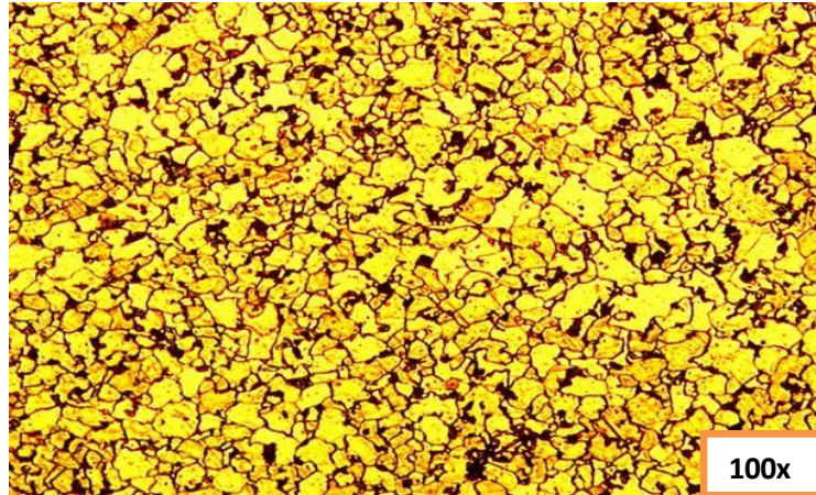
Figure 6 Transverse cross-sectional micrograph showing ferrite & pearlite.
