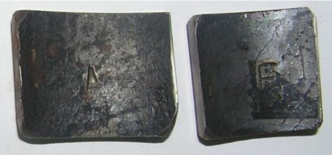
Figure 4 Oxide layer (scale) on the inner surface of sample A & F
