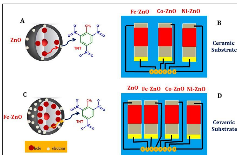
Figure 3 Fe-doped ZnO chemiresistive sensor (A and C) Models showing the charge transfer mechanism of undoped and doped ZnO (B) Schematic representation of the gas sensor array composed of three doped sensor; Fe-ZnO, Co-ZnO and Ni-ZnO, (D) Schematic representation of the gas sensor array composed of four sensor; ZnO, Fe-ZnO, Co-ZnO and Ni-ZnO.[29]
